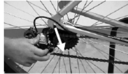
With the derailleur pulled back, space is created for the wheel to be removed
